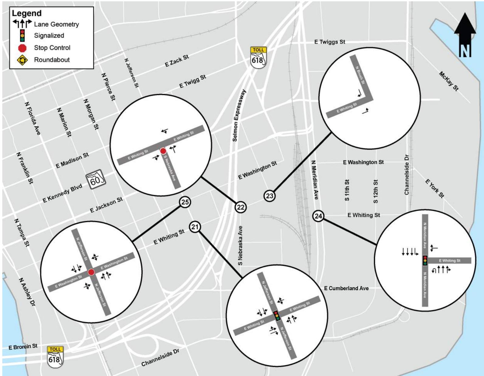
Figure 2.2e: Existing (2019) Lane Geometry
