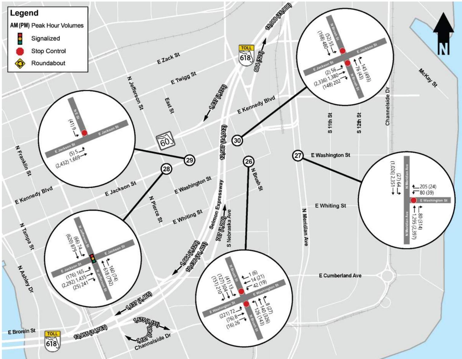
Figure 4.9f: Design Year (2046) No-Build Alternative Turning Movement Volumes
